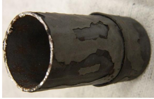
Fig 9. Pitting Corrosion on the Inner Surface and FeO (the layer adjacent to iron), Fe 3 O 4 (middle layer) and Fe 2 O 3 (surface layer), on the Outer Surface.
