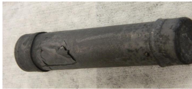
Fig 8. Steel Canister with End-caps Sealed with Sodium Silicate and Filled with PCM, after 10 Thermal Cycles.
