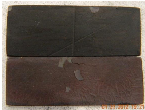
Fig 18. Steel Sample Heated to 700 • C Top: With Sealmat Coating No Scaling, Bottom: No Coating Forms Scales
