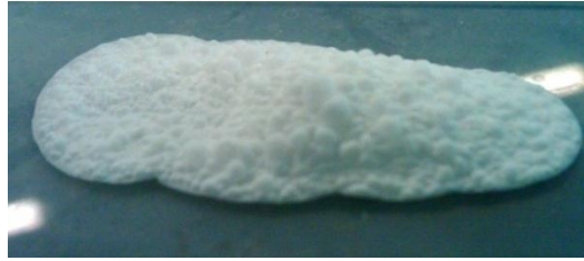
Fig 10. Sodium Silicate Cured on Glass at 300 °C, Forms Efflorescence
