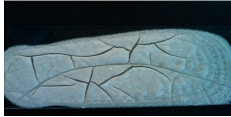
Fig 12. Sodium Silicate Coating on Glass Cured at 200° C on a Hot-plate Displays Cracking
